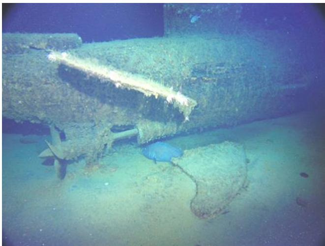
HMAS AE1 - starboard propeller, after hydroplane, hydroplane guard and resident grouper.
