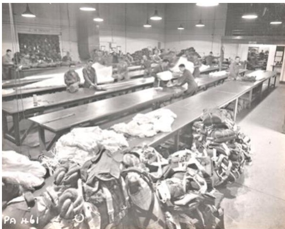
Shown is a photo of the parachute shop at Burtonwood, England, Depot Hundreds of parachutes can be seen in the photos. Seat-pack, back-pack and Quick Attachable Chest parachutes are present. In the foreground a drop test dummy with an OD A-3 harness is present. On the tables parachutes can be seen in various states of packing.
